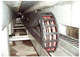
The main trolley on the new STS cranes travels at a speed of 13 ft/s (4 m/s). igus<sup>®</sup> Rol-Energy Chain<sup>®</sup> roller cable carriers are used for data and energy transmission. In this high-speed application, it is not necessary to use additional control or drive systems for the cable carriers. Another advantage compared to conventional systems is the weight reduction in the trolley drive system and crane carriage.
